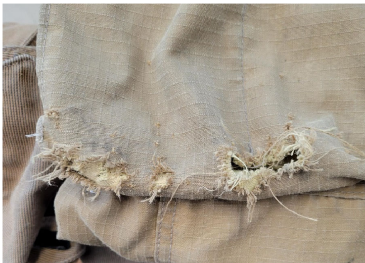
(Above: PPE Pants with holes worn through the fabric.)
